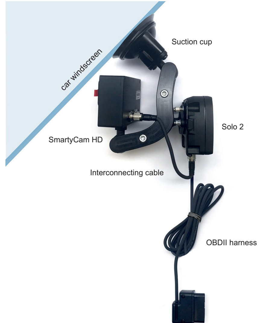
Pic 5: Cable connection on final layout
