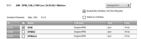
Select the desired RPM multiplier factor, in dependence upon your engine and the number of sparks per revolution.
