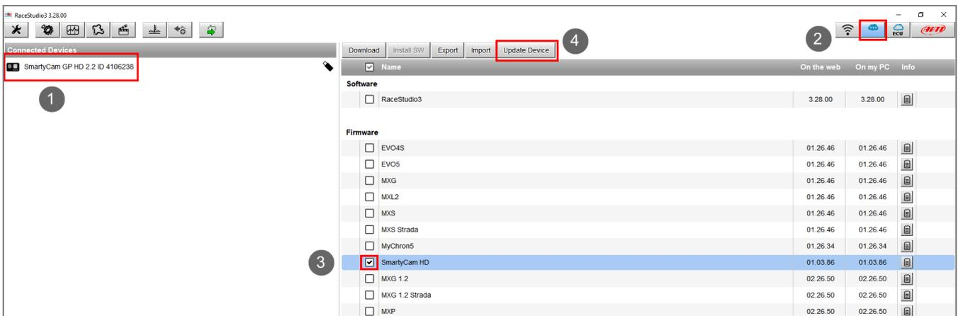
At the end of the updating, SmartyCam automatically resets itself, then firmware upgrade process starts ("Smarty upgrade is starting: DO NOT POWER OFF THE SYSTEM!), then press any key to switch SmartyCam on normally.
