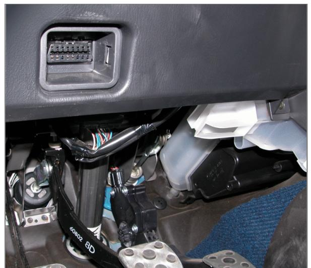
The ECU communicates using the K line on the OBDII connector. Connector pinout as well as connection table are shown here below.
