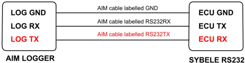
**Note: Sybele Challenge RS232 needs connection of LOG TX cable to ECU RX pin too.**
