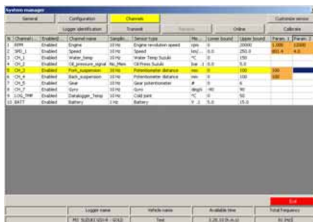
Figura 29: Race Studio 2 Finestra canali in ingresso (channels).
