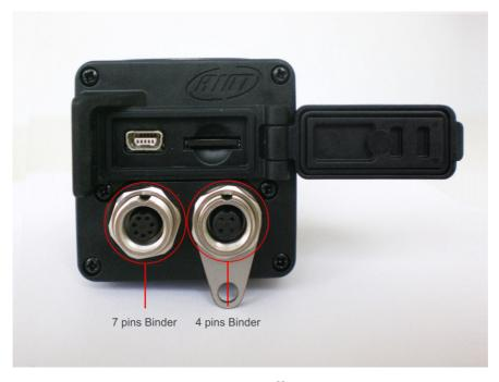
SmartyCam stand alone can be connected in different ways:
