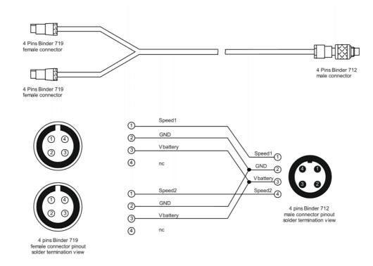
**MXL Strada**/**Pista** have one only speed channel. Speed sensor is included in the optional basic sensor kit – part number **X10MXLS00000** – that includes RPM and water temperature sensors too. The cable part number is: **V02554020**.
