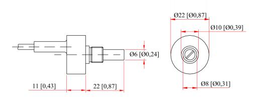
The following images shows the pulleys dimensions in millimetres [inches]:
