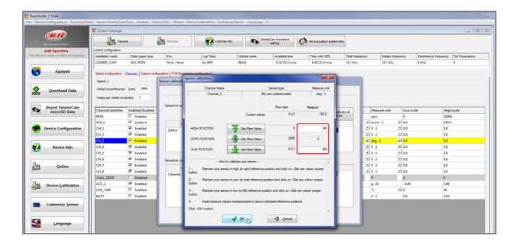
swerve to the right according to the angle you wish to calibrate and press "Get raw value" corresponding to "High position"
