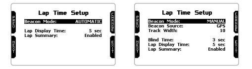
In **automatic mode** MyChron5 recognizes if an optical/magnetic receiver is connected in addition to the integrated GPS. In this case both receivers work at the same time continuously exchanging and comparing information about track finish and split points you cross. You can:
