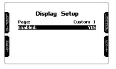
Each custom page can show up to four fields. Pressing "SELECT" you can choose the channel to show in each field. The only field that can show lap time in different formats is bottom right one (right image below).
