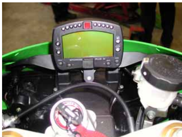
Figure 10: MyChron 3 Plus correctly installed.
