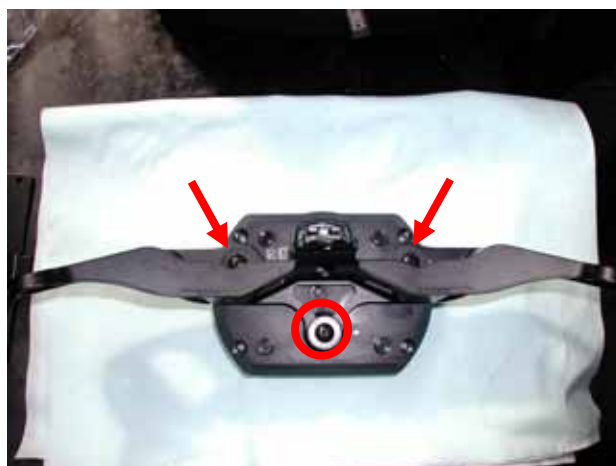
Figure 6: screws that fixes the stock dash
