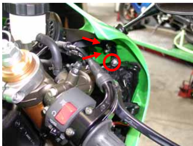
Figure 3: Lateral mirrors screws.
