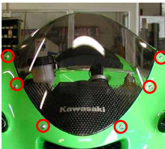
Figure 1: front transparent fairing – screws location
