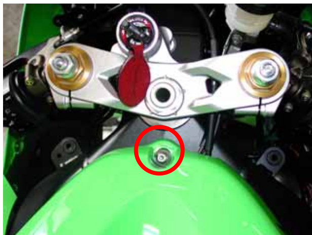
Figure 14: location of the gas tank screw
