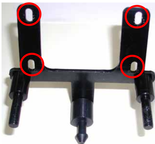
Figure 7: Anchor plugs are fixed to the bracket
