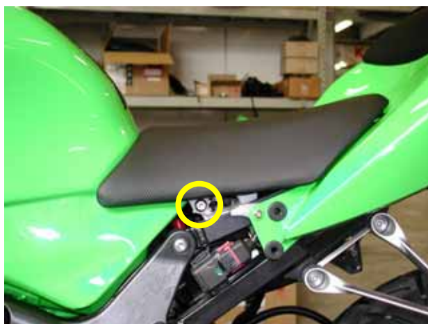
Figure 13: the screw that fixes the seat to the bike.
