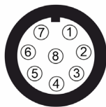
8 pins Binder 712 female connector pinout front view
