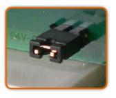
The image here above on the right shows possible working mode. The transmitter comes set in low power mode: see images on top on the right. To set high power mode insert both clips in the jumper: image bottom on the right.
