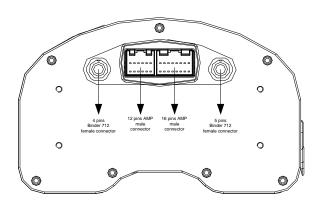
4 pins Binder 712 female connector pinout - Beacon
