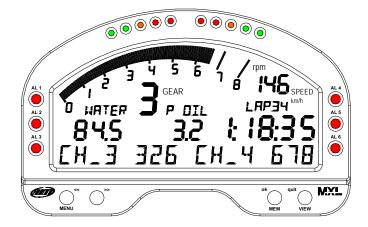
The ten top led (shift light) of the display are connected to engine RPM; values corresponding to each led are set via software or via keyboard. See the paragraph concerning keyboard function or **Race Studio Configuration** user manual for further information on the subject.
