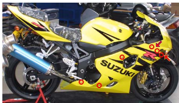
Figure 4: right lateral fairing – screws and pins.
