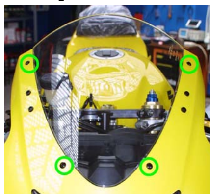
Figure 3: front screen – 4 Phillips thread forming screws.
