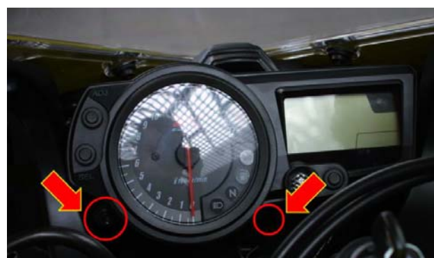
Figure 14: stock dash front screws position.
