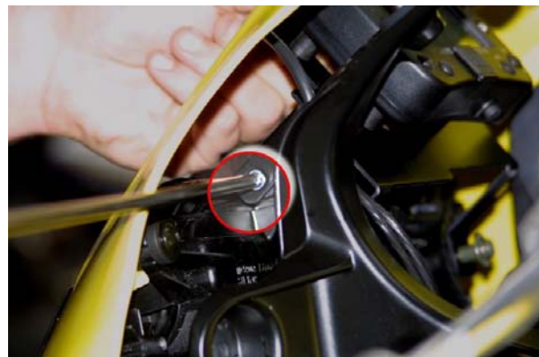
Figure 29: lateral screws fixing
