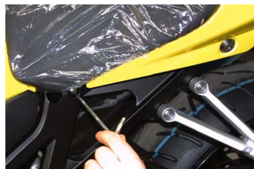
Figure 9: unscrew the bike screws
