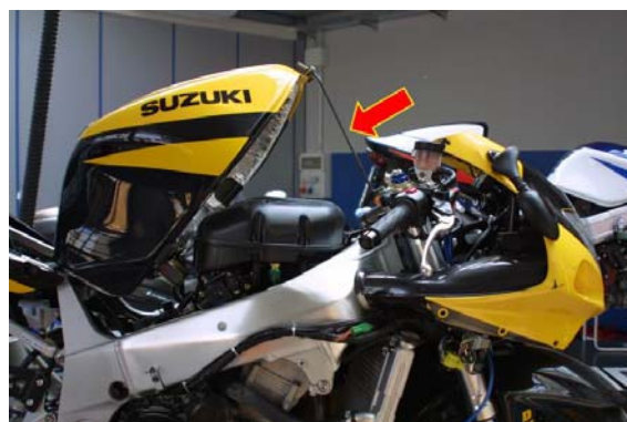
Figure 11: lifting the fuel tank
