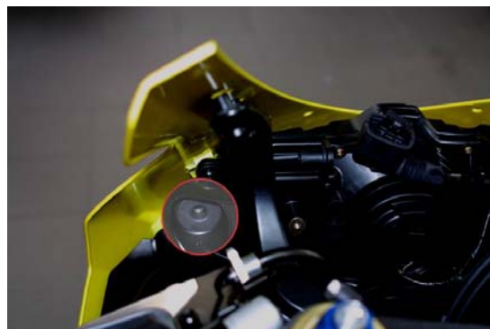
Figure 12: front fairing and high beam screws position
