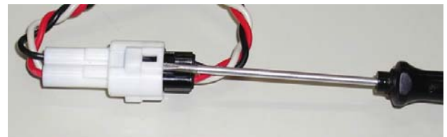
Figure 20: how to unplug a connector.
