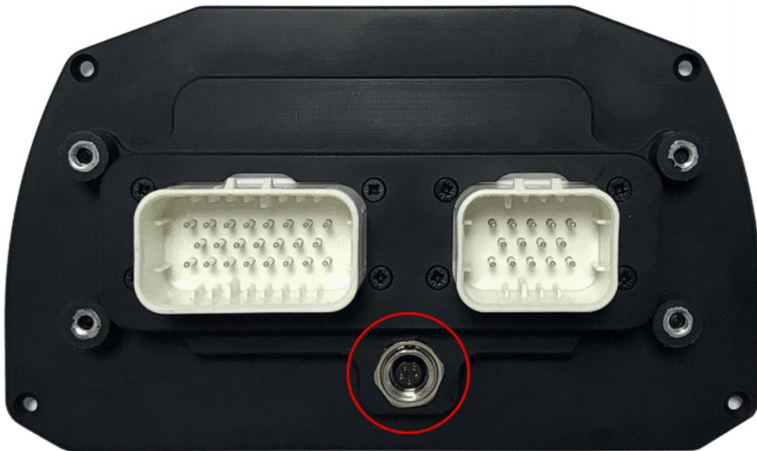
Rear cameras need to be connected to the logger, set in the logger configuration through Race Studio 3 software and executed through the logger keyboard. Here follows explanation of how to perform all these operations.
