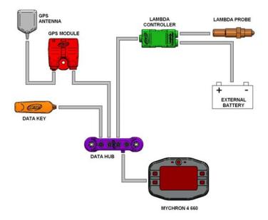
Though the system is powered through Lambda controller connected to the battery, it is suggested to leave **MyChron4 660** internal batteries in the logger. Lambda controller switches automatically off when **MyChron4 660** is switched off.
