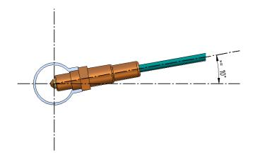
Once installed the probe, please pay attention not to let the cable pass near to excessive heat sources (the exhaust pipe for example).
