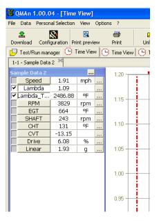
To better analyse carburettor values we would suggest you to show XY diagram of Lambda probe with RPM values on abscissa axle and Lambda values on ordinate axle on the graph.
