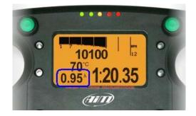
Switching **EVO3** on, Lambda controller is recognised at start up and probe Warm-Up procedure starts. During this period the controller takes the probe to its working temperature (until around 780  $^{\circ}$ C – 1436  $^{\circ}$ F).
