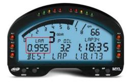
Switching **MXL** on, Lambda controller is recognised at start-up and probe Warm-Up procedure starts. During this period, the controller takes the probe to its working temperature (until around 780  $^{\circ}$ C – 1436  $^{\circ}$ F).
