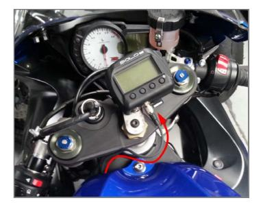
To connect SoloDL to male Binder connector of **V02569140** use the 7 pins female Binder connector placed bottom right of the logger as shown here below.
