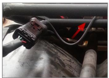
To reach SoloDL make the cable pass between the fuel tank and the bike frame.
