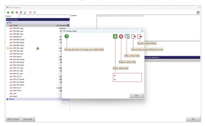
LookUp table is a special function of Race Studio 3 Analysis whose working mode is very close to what custom sensors do for the configuration. You can define a "curve" according to which, given the value of one or two channels, you define the output value. Look up table can be:
