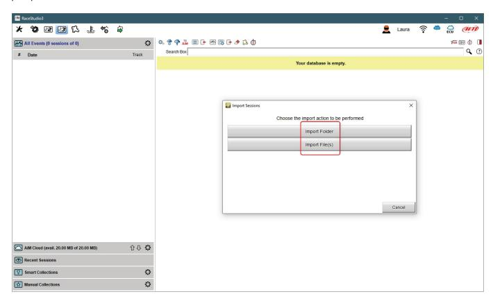
It is possible to import single files or entire folders of data. Pressing one of the buttons highlighted browse windows is prompted: select the file/folder to import and press OK. A panel with a progress bar appears. In case the files are already in the database or if there is any issue the software warns you.
