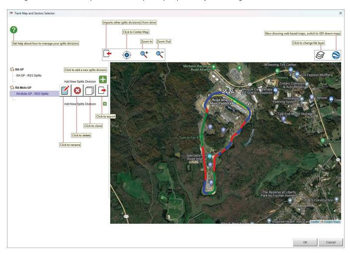
As for any track map you can import the split division from the device, centre and zoom it in/out using the top left keyboard as well as decide the map tile provider and switch among web mapping and GDI drawn map using the top right keyboard.
