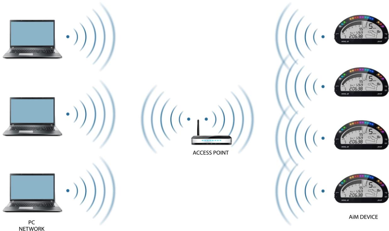
In this configuration both your AIM device and your PC have to join a pre-existing Wi-Fi network, called WLAN, in order to communicate with one another. The network is now created by a network device which is acting as an external Access Point permitting the device connectivity.
