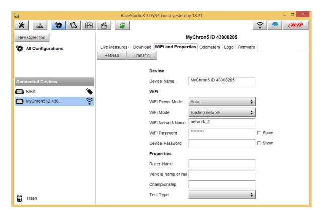
As you can see by the picture previously reported, the device called "MyChron5 ID 43008208" is switched from AP mode to WLAN mode. The network name is "network\_2" and it is not working in open authentication mode since protected by a network password.
