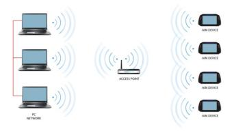
In this configuration, both your AIM device and your PC have to join a preexisting WiFi network, called a WLAN, in order to communicate with one another. The network is now created by a network device which is acting as an external Access Point by permitting the device connectivity.
