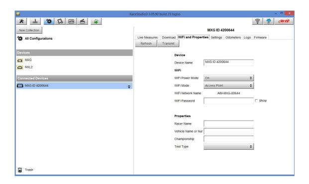
When initially configured as an Access Point, your AiM device creates a network without a password that is accessible to everyone. It is therefore recommended that you create a unique password to secure your device/network immediately. With the use of a password, the communication is secure and encrypted using the WPA2-PSK standard.
