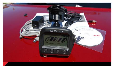
The AiM Solo comes with all of the items shown here to make your experience a satisfying one. A car charger complements the built-in battery and charger, and the USB cable makes downloads to your computer simple. The user manual and analysis software CD will get you up and running quickly. The Solo DL will allow connection to your car's OBDII data stream and a SmartyCam video camera.
