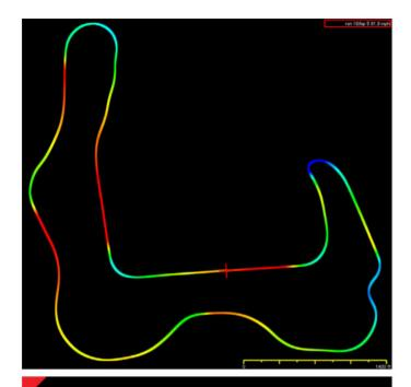
This Solo GPS-generated track map is color coded with speed, so the speed data is easy to see and understand. The speed spectrum colors are in the order of a rainbow, with blue as slow and red as fast.
