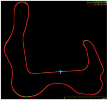
Overlaying maps from two different laps shows differences in lines. This can help you learn why the lap shown in green was faster than the early lap shown in red. The color of each lap is automatically displayed in a different color to make comparisons easy.
