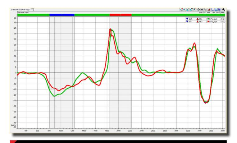
This display shows only a portion of the lap for more detailed analysis. Zooming in like this is very simple in Race Studio Analysis. The data displayed here is the turn rate of the car in degrees per second. Nazarian rotated the car much more quickly at the entry and exit of Turn 1. The crosshair is shown at the peak of the yaw rate, which was 21.0 degrees per second turning to the left. This zoomed-in view shows that the rate of data sampling is high enough for analysis in fine detail.
