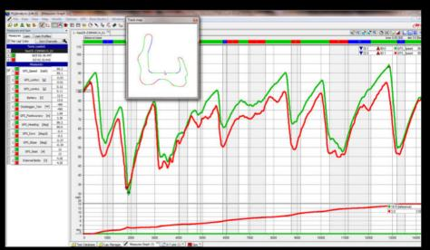
trace at the bottom of the screen is the difference in elapsed time to each point on the track. This data shows exactly how and where a 7 mph speed difference throughout a lap added up to a 14-second lap time difference. This kind of information is highly valuable for driver development and car setup development.
