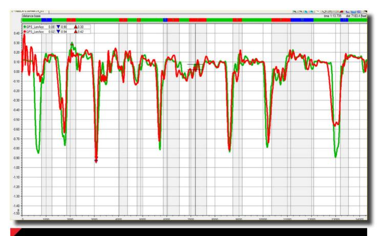
The longitudinal acceleration comparison of these two laps shows that Nazarian consistently braked later and harder during the faster green lap.
