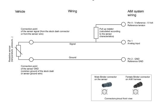
If the fuel level signal is taken from the original dashboard connector, it is possible that the sensor ground wire (GND) is not available: in this case connect the common ground of the vehicle connector to one of MXS Strada analog ground inputs or to pin2 of one of the Binder connectors dedicated to MXS Strada analog inputs on 23 pins connector optional harness.
