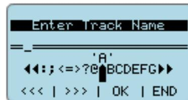
If the track is stored in the logger memory (“Select”) just select it, if not (“Enter Names”) place the slider on an empty position (or the system overwrites the one stored) and press “OK”. “Enter track name” page opens. Once the name composed press “OK”. The system asks for confirmation, press “Yes”. The system can store up to 50 circuits.
