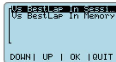
In both cases an under menu opens: it is possible to compare lap time with the best lap in the session or with the best lap recorded on that track (Vs Best Lap in memor...). In this second case it is necessary to have previously set the track.
