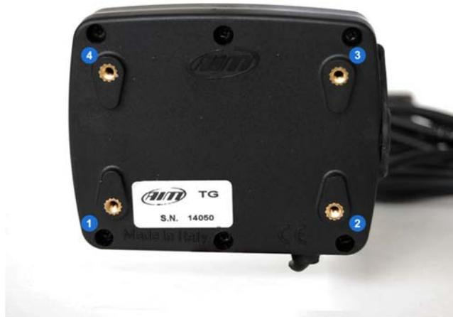
**MyChron Light TG** is powered by two 3 Volts round batteries type CR 2430 included in the infrared receiver. To change the batteries see the chapter concerning **MyChron Light TG** maintenance.
