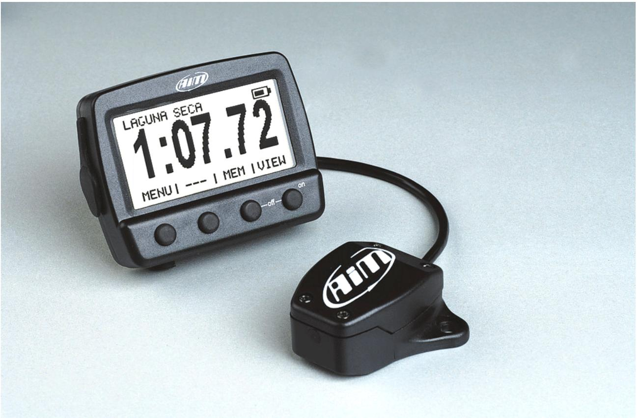
**MyChron Light TG**, the new AIM lap timer, is the evolution of the well known MyChron Light MCL. This new logger merges all functionalities and good qualities of its forefather with the new graphic display and adds a lot of other useful functions, like the visualisation of sampled data as histograms and the different working and sampling modes.
