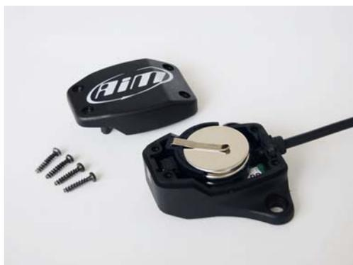
**MyChron Light TG** uses two 3V round batteries code CR2430. The code is generally stamped on the batteries.
