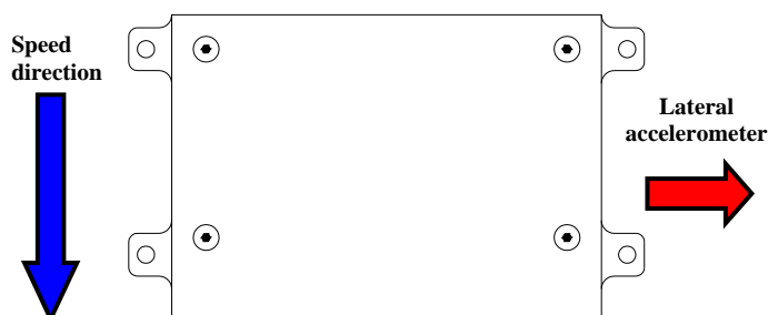
Figure 3: How to correctly install your MyChron 3 XG (Junction box’s top side view)
