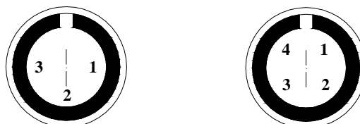
3 & 4 pins female Binder 712 connectors pinout: external view
