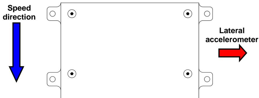
In order to correctly measure the lateral g-force using the internal accelerometer, it is recommended to install the gauge with the Junction box's front panel perpendicular to the vehicle's speed.
